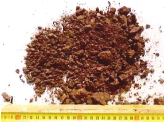
A photograph of a dark brown, granular soil sample from borehole T2 at 0.7m depth. The sample is irregularly shaped and contains visible rock fragments. A yellow metric ruler is placed horizontally in front of the sample for scale, showing centimeters from 0 to 30. |
