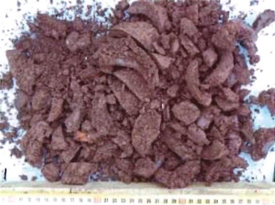
A photograph of a dark brown, crumbly soil sample from test T6. The sample is irregularly shaped and sits on a white surface. A yellow metric ruler is placed horizontally in front of the sample for scale, showing centimeters from 0 to 30.                                                     |
