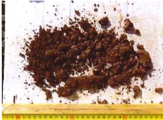
A photograph of a dark, moist soil sample, likely argillic or limonitic, resting on a white surface. A yellow metric tape measure is visible in the background for scale. |
