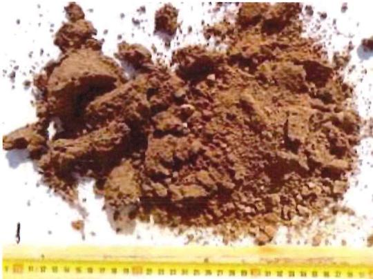
A photograph of a dark brown, granular soil sample from borehole T1 at 0.6m depth. The sample is irregularly shaped and contains visible rock fragments. A yellow metric ruler is placed horizontally in front of the sample for scale, showing centimeters from 0 to 30.  |
